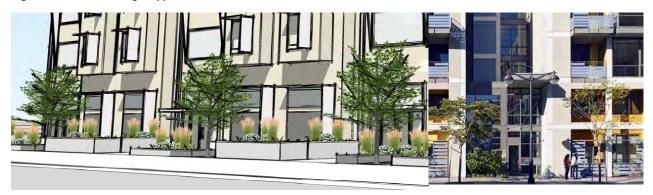
c) Arcade/Gallery Frontage Type: Arcades are a Flex Frontage type where façades have an attached colonnade covered by upper stories. This type is ideal for future uses on the west side of 132<sup>nd</sup>. For Building Code considerations, this frontage type cannot cover the public right-of-way.
