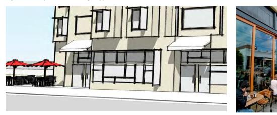
b) Flex Front Frontage Type: Flex Frontages are designed so that ground floor retail and commercial uses may be used for temporary residential uses, and uses may be interchanged. The design flexibility allows for ground floor façades to transition between shop front requirements and residential uses.
